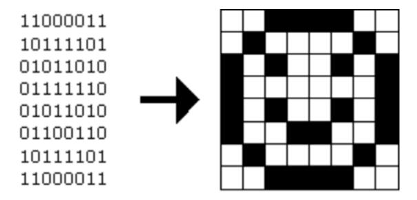
In this sense, then, is an image just a bitmap (i.e., a map of bits). For more colorful images, you simply need more bits per pixel. A file format (like GIF) that supports "8-bit color" uses 8 bits per pixel. A file format (like BMP, JPEG, or PNG) that supports "24-bit color" uses 24 bits per pixel. (BMP actually supports 1-, 4-, 8-, 16-, 24-, and 32-bit color.)
