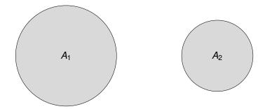
$A_1$  is twice the area of  $A_2$ . For simplicity, let's assume that the diameter of  $A_1$  (which we'll call  $d_1$ ) and its focal length (*f*) are both 1, so the F-number of this lens would be 1. Let us further assume that the focal length of the lenses are the same. To figure out the F-number of  $A_2$ , we need to determine how much smaller the diameter is compared to that of  $A_1$ . Let's do some math!
