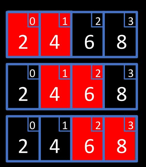
initialize counter do { set counter to 0 iterate through entire array if array[n] > array[n+1] swap them increment counter while (counter > 0)
